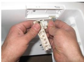
Remove the Led-Board and pull out the data cable.
